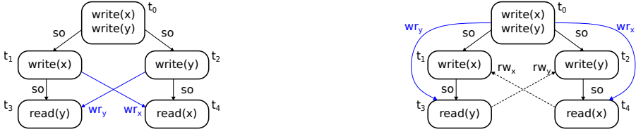
(a) An observed execution for which a CAUSAL, UNSERIALIZABLE predicted execution exists.
